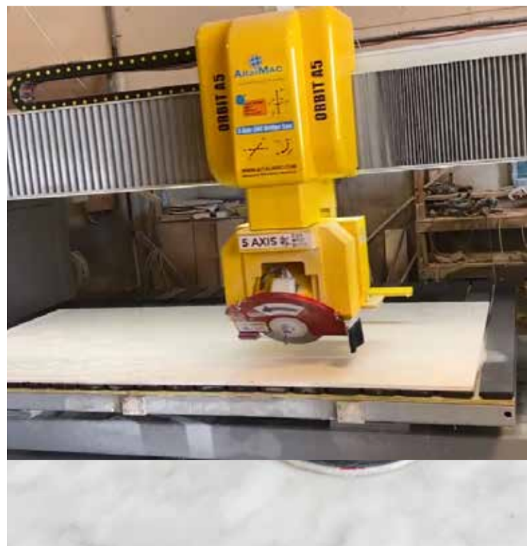
Image: AitalMac 5-axis CNC Bridge Saw Orbit A5 machine at our Richmond Factory
